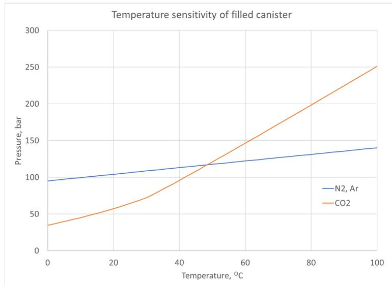
To maximize the value of the constant pressure characteristic of a dual phase gas, it is important to minimize the “dead volume”. In this way, there is less expansion upon initial release of gas from the cylinder and the pressure can be held constant through the greatest working volume change possible.
